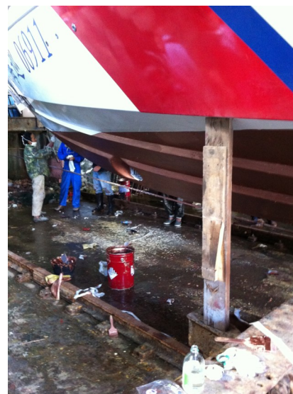
View on the ship's hull coated with Humidur®
