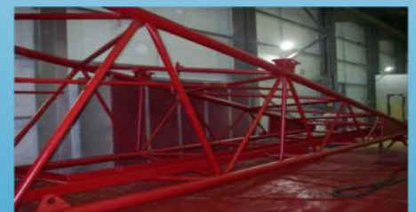
Offshore crane structure
