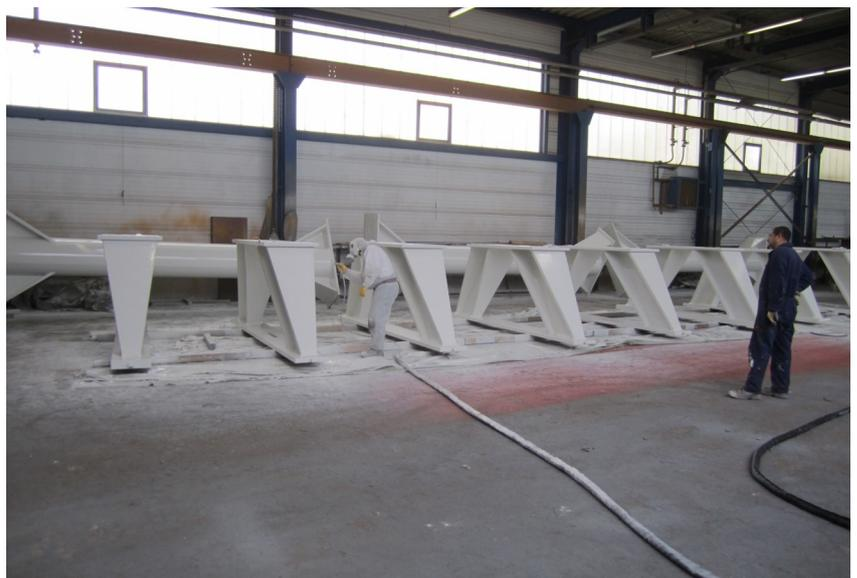
Finished section with Humidur light grey
