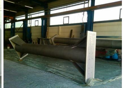
Different parts in warehouse after surface preparation to near white steel (Sa 2,5)
