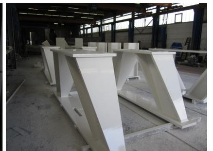
Coating of Humidur on near white steel and on top of welding primer (pictures above)
