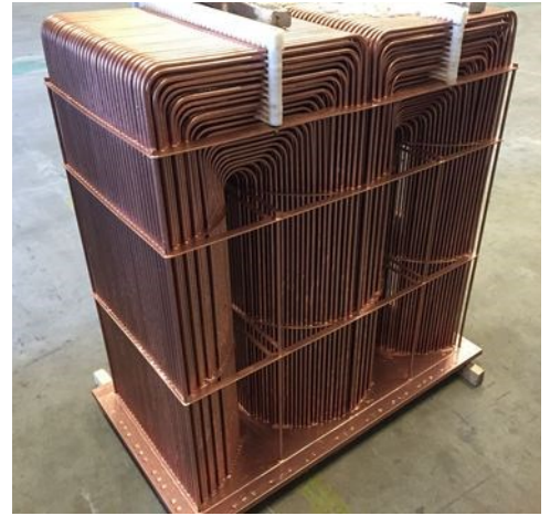
Box cooler coated with Humidur AF
