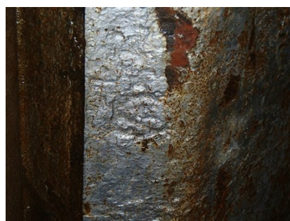
Pitting due to MIC in submerged zone
