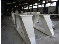
Coating of Humidur on near white steel and on top of welding primer (pictures above)
