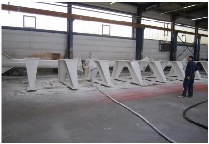
Finished section with Humidur light grey
