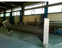
Different parts in warehouse after surface preparation to near white steel (Sa 2,5)
