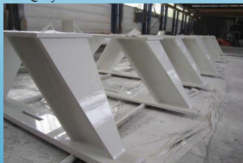
Steel supporting parts in subway stations
