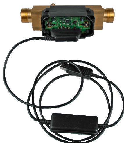
Figure 28. Location of the four-pole plug in ULTRAFLOW® 54.
