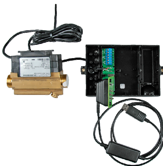
Figure 29. Location of the four-pole plug incl. ULTRAFLOW® 14 adapter in ULTRAFLOW® 14/24 (MULTICAL® 61/62).
