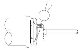
Sealing of ø5.8 mm temperature sensor mounted in pocket, type number 6557-324.
