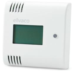
The CMa10w is a wireless M-Bus communicating temperature and humidity sensor for indoor use. CMa10w complies with the OMS standard and operates in wireless M-Bus mode T1. CMa10w is easy to install, has a high accuracy and long life time, which make it the perfect choice for tenant owners when wiring is not an option.
