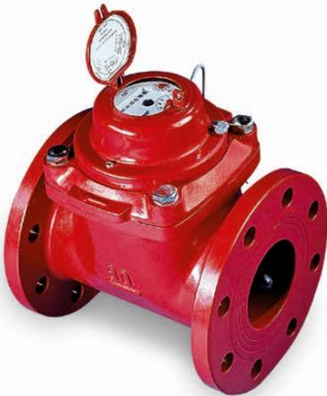
Woltman Parallel type meters are always used when high flow rates with a relative constant flow rate profile are to be measured. Through its robust construction they not only are capable of covering a large measuring range, but the measuring accuracy is also long-term stable.
