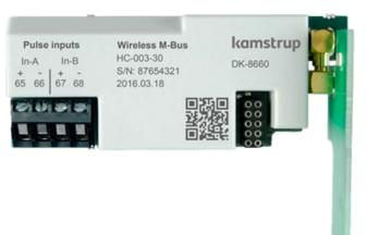
A large selection of datagrams for various applications can be configured into the Wireless M-Bus module.
