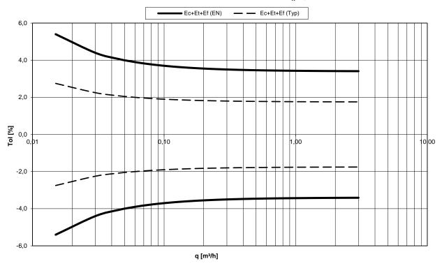
Diagram 1: Total typical accuracy of MULTICAL® 603 and ULTRAFLOW® compared to EN 1434-1
