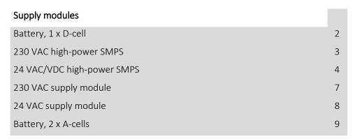
All supply modules have been evaluated in connection with the extensive type tests, to which MULTICAL® 603 has been subjected, and it is not permissible to use other supply modules than the ones mentioned above. The supply modules are covered by the CE-marking and the factory guarantee of the meter.
