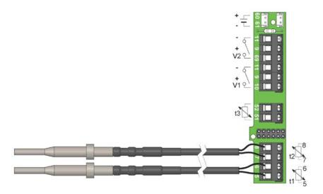
Cable lengths and cross sections of the two sensors which are used as temperature sensor pair for a heat meter must always be identical, and cable sensors must neither be shortened nor extended.
