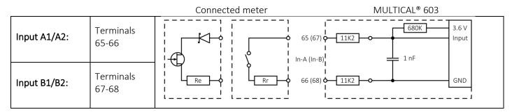
The pulse inputs are configured as a part of the meter's configuration number via the FF and GG codes. Upon receipt of order, the FF and GG codes are configured at 24 by default (unless otherwise informed by the customer). Valid FF and GG codes appear from the table below. The default code 24 is marked in green. The FF and GG codes can be reconfigured by means of METERTOOL HCW. See Technical Description for METERTOOL HCW (5512-2097).
