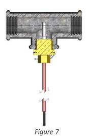
As it appears from Figure 7, the short direct sensor DS 27,5 mm can be mounted by means of an  $R\frac{1}{2}$  or  $R\frac{3}{4}$  for M10 nipple in a standard 90° tee.
