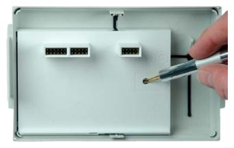
It is recommended to complete the work in the TEST loop before starting the reconfiguration via the SETUP loop or METERTOOL as every reconfiguration is logged in MULTICAL® 603 (it is only possible to reconfigure MULTICAL® 603 50 times).
