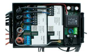
Wireless M-Bus-module with internal antenna
