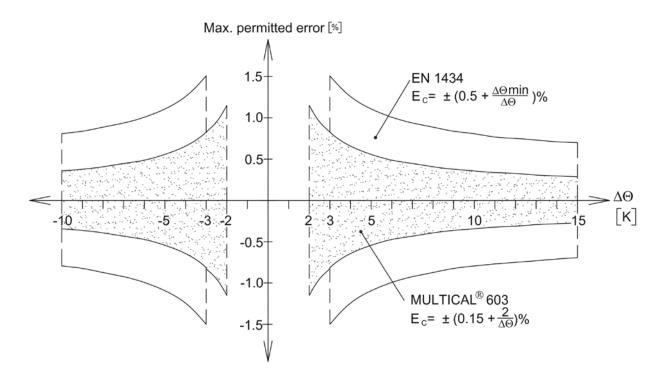
Figure 2: Typical accuracy of MULTICAL® 603 compared to EN 1434.
