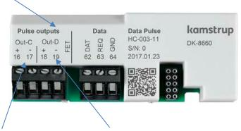
Terminals for Out-C and terminals for Out-D are marked as well.
