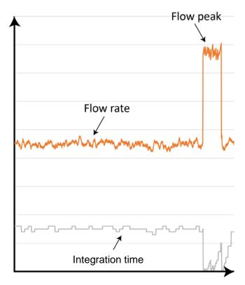
Thus, in adaptive mode MULTICAL® 603 measures at high resolution during periods with changes in the system requiring accurate measurements and saves battery power during periods with no changes in the thermal system.
