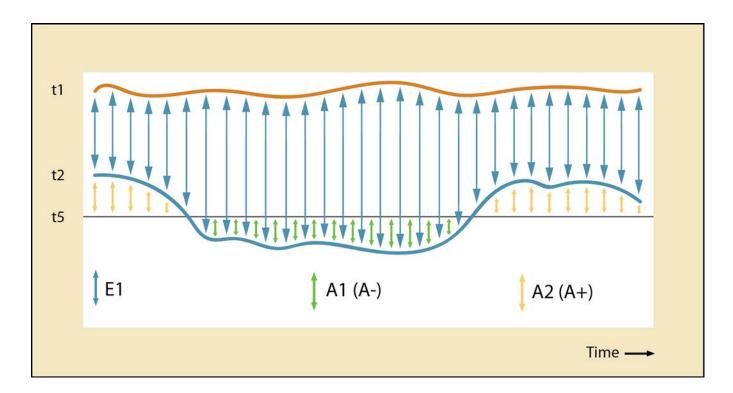
The outlet temperature reference t5 can be factory-configured as required, or can be changed via METERTOOL HCW after delivery. Typical configuration is t5 = 50 °C.
