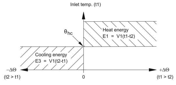
$\theta_{hc}$  functions as a limit value for the measurement of heat/cooling energy. With  $\theta hc$  enabled, heat energy is only measured when t1 is greater than or equal to  $\theta_{hc}$ . Likewise, cooling energy is only measured if the inlet temperature t1 is lower than  $\theta_{hc}$ .
