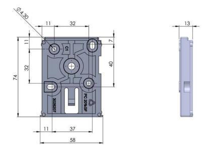
Figure 6: Wall bracket, 3026-207 for MULTICAL® 603
