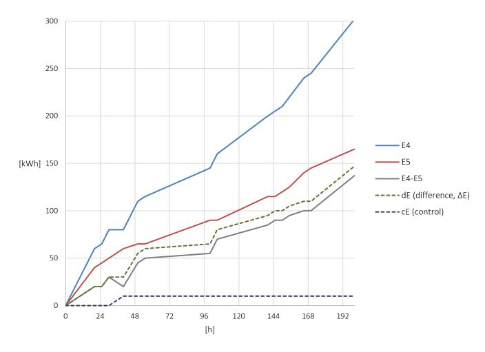
In a scenario where no counting is taking place in register E4 (energy fed), e.g. due to air in flow meter V1, the counting will take place in cE (control). This is shown in the above example between data items 24 and 48 [h].
