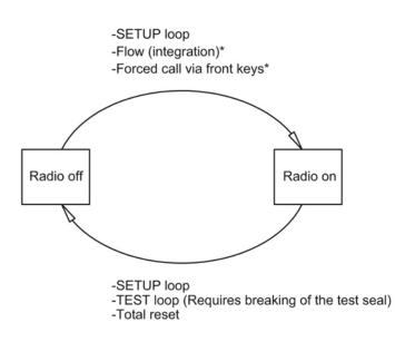
\*If the meter is in TEST loop the radio remains off at flow (integration) and forced call
