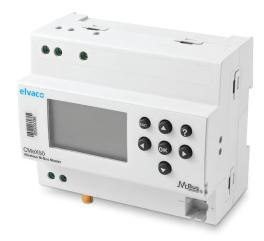
CMeX50 is a wireless M-Bus master which can be used by any existing wired M-Bus solution or together with Elvaco CMe Series products. The CMeX50 communicates with wireless M-Bus slaves via the wireless modes S1, S2, T1, T2, C1 and C2, and is compatible with all widely used M-Bus slaves on the market. The CMeX50 handles up to 500 wireless M-Bus slaves, which can be individually secured by encryption keys. It also has a built-in M-Bus master for 32 wired M-Bus slaves.
